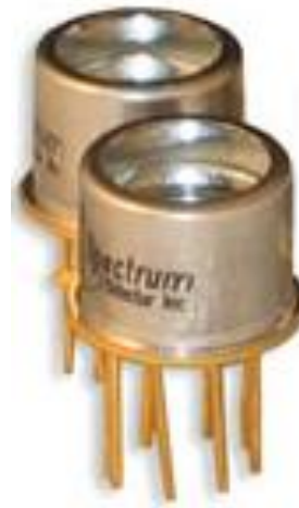
Figure 5. SPC-2 Lithium Tantalate pyroelectric sensor.
